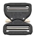
The COBRA® PRO STYLE is the world leading safety buckle made of aluminium. Thanks to its patented locking mechanism and high breaking strength it meets the highest safety requirements. In combination with a fitting webbing, the minimum guaranteed load capacity is 9 kN tensile strength and 18 kN in loop configuration.
