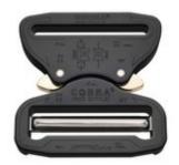
The COBRA® PRO STYLE is the strongest and world leading safety buckle made of aluminium. Thanks to its patented locking mechanism and high breaking strength it meets the highest safety requirements. In combination with a fitting webbing, the minimum guaranteed load capacity is 9 kN tensile strength and 18 kN in loop configuration.
