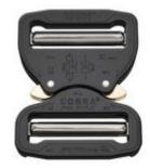
The COBRA® PRO STYLE is the strongest and world leading safety buckle made of aluminium. Thanks to its patented locking mechanism and high breaking strength it meets the highest safety requirements. In combination with a fitting webbing, the minimum guaranteed load capacity is 9 kN tensile strength and 18 kN in loop configuration.
