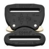
The COBRA® PRO STYLE is the strongest and world leading safety buckle made of aluminium. Thanks to its patented locking mechanism and high breaking strength it meets the highest safety requirements. In combination with a fitting webbing, the minimum guaranteed load capacity is 9 kN tensile strength and 18 kN in loop configuration.
