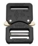
The COBRA® PRO STYLE is the strongest and world leading safety buckle made of aluminium. Thanks to its patented locking mechanism and high breaking strength it meets the highest safety requirements. In combination with a fitting webbing, the minimum guaranteed load capacity is 9 kN tensile strength and 18 kN in loop configuration.
